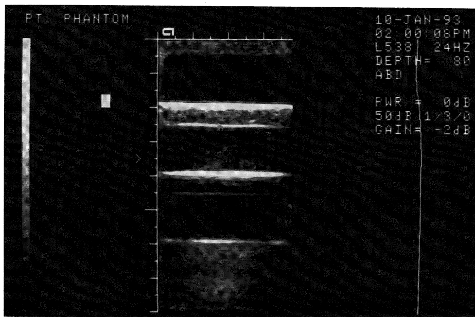
Figure 3. The image produced by an Acuson medical imaging device using the experimental wax/water phantom described in the text.
